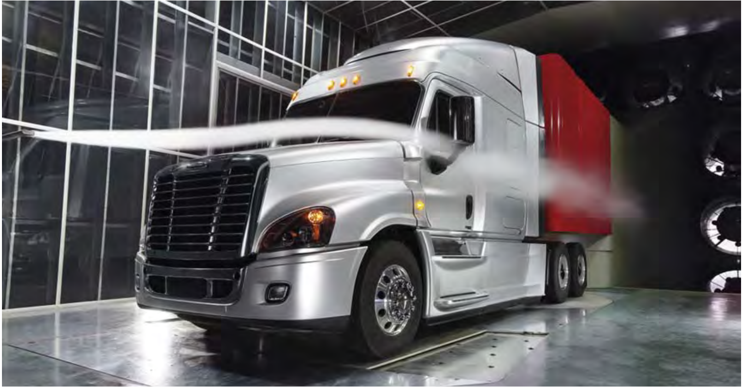
The Freightliner Cascadia Evolution offers fuel savings of seven percent, thanks to aerodynamic improvements and the new Detroit DD15 engine with Daimler BlueTEC exhaust treatment technology.
